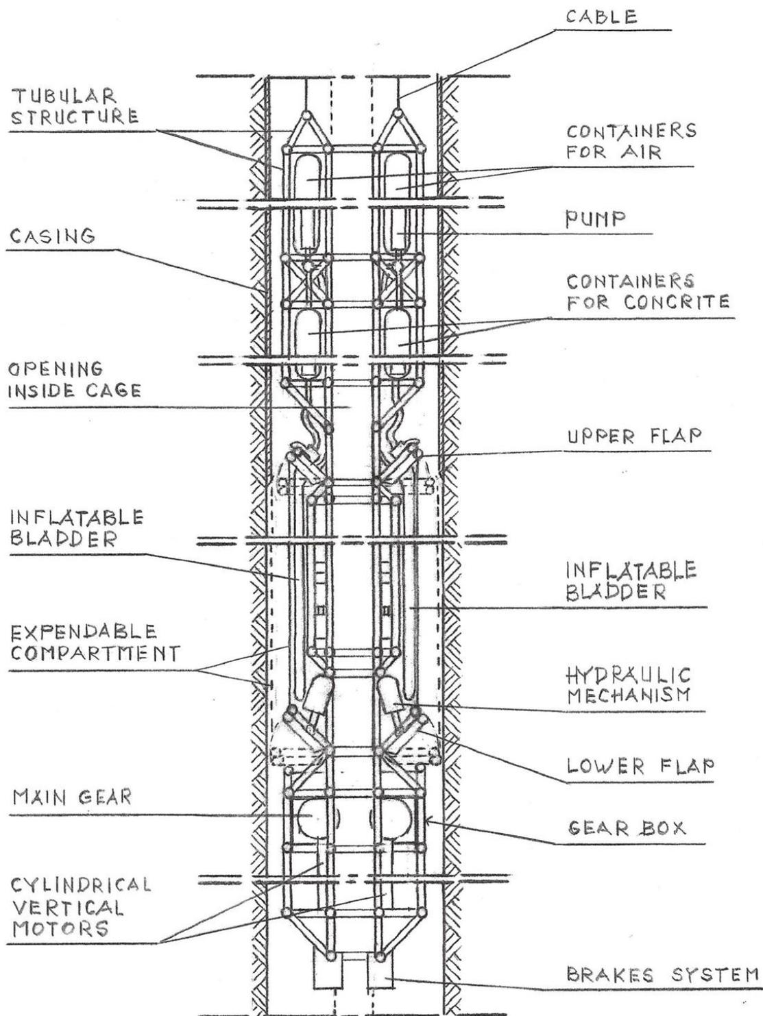
**Figure 7:** Cross-sectional View of an Circular Cage to be assembled on the Excavation Line of the apparatus for Drilling Faster, Deeper, and Wider Wellbore.
