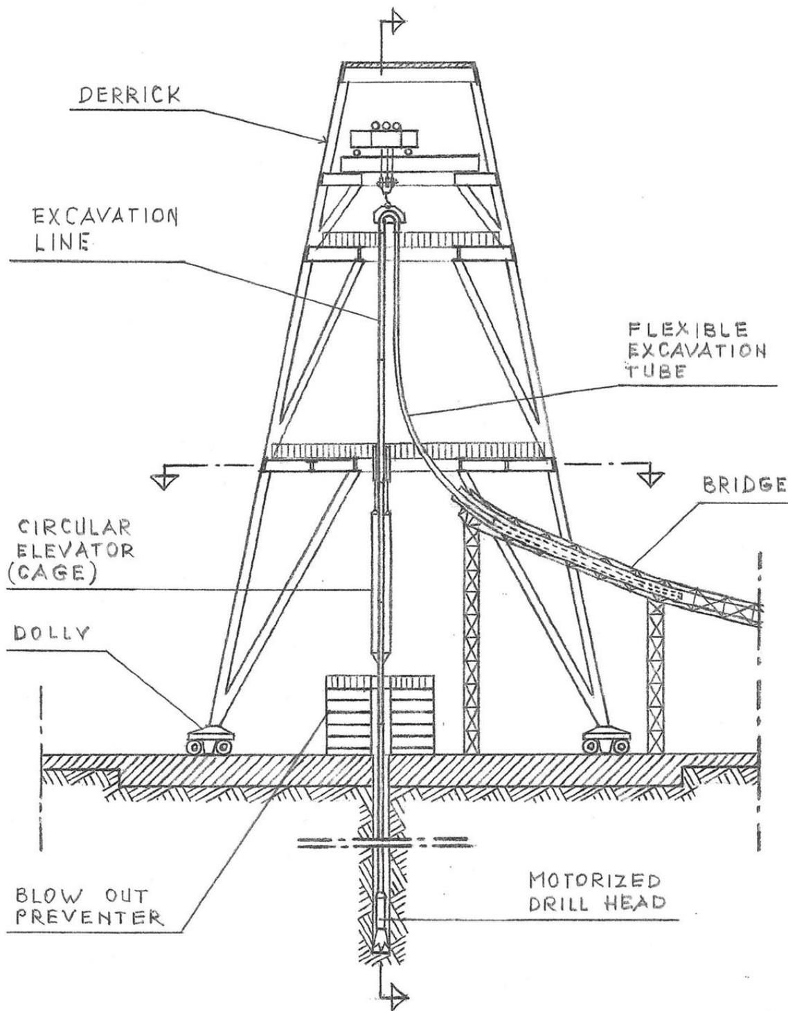
**Figure 3:** Another Schematic View of an Apparatus for Drilling Faster, Deeper, and Wider Wellbore with a Cage for Casing
