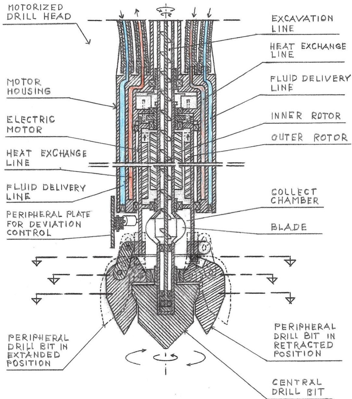
**Figure 7:** Cross-sectional View of the Motorized Drill Head for Drilling Faster, Deeper, and Wider Wellbore
