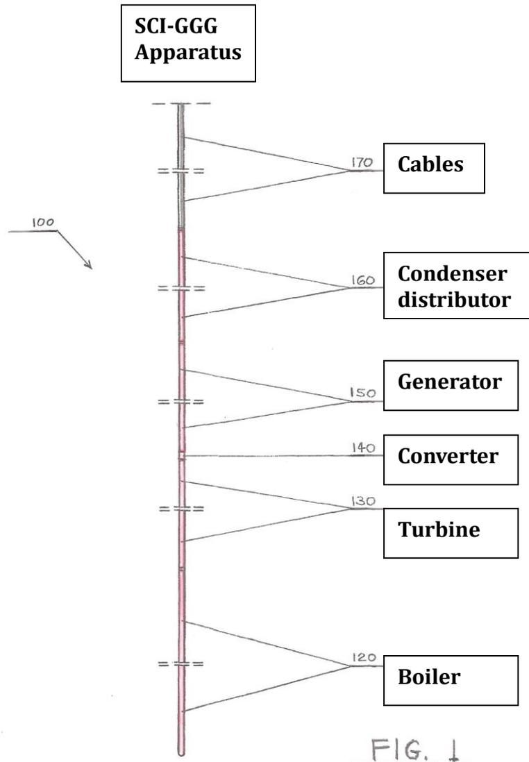
The SCI-GGG system uses several completely closed loop systems and generates electricity down at the heat source and transmits it up to the ground level by means of electrical cables.
