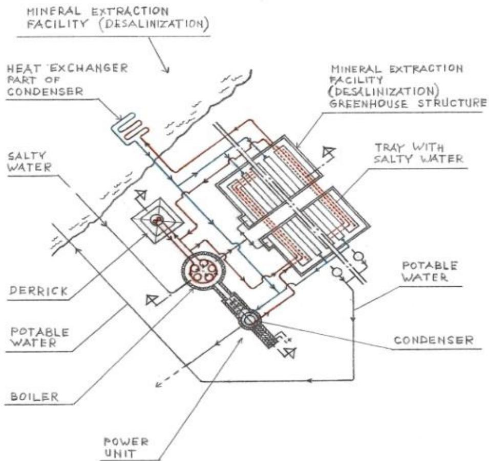
**FIG. 16 – Schematic Plain View of a Power Plant for Desalinization of the Salton Sea, Production of Electricity, Potable Water, and Lithium**
