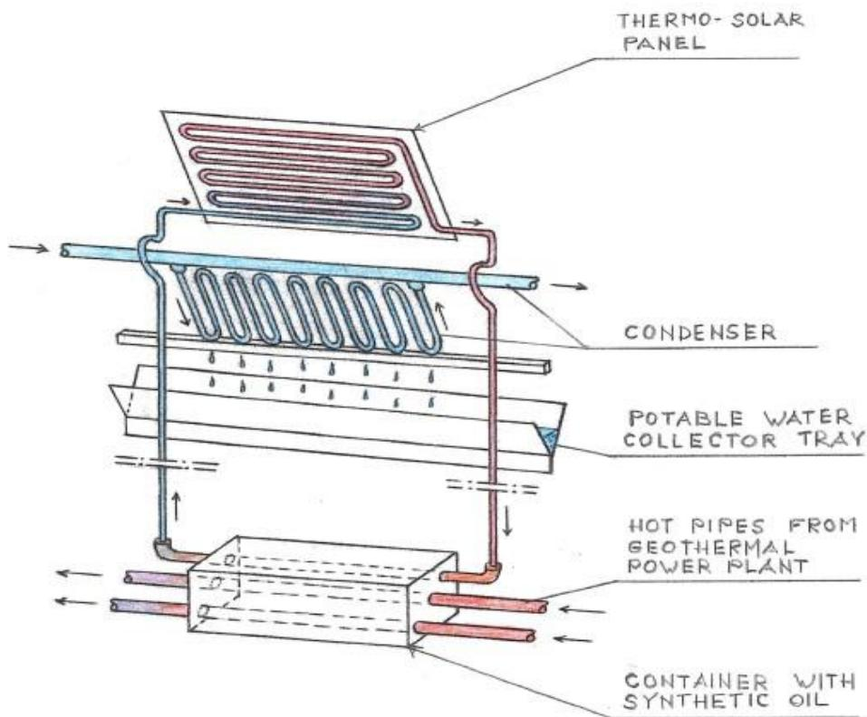
**FIG. 18 – Perspective Cross-sectional View of an alternative Thermo-Solar System used in Desalination Plant**
