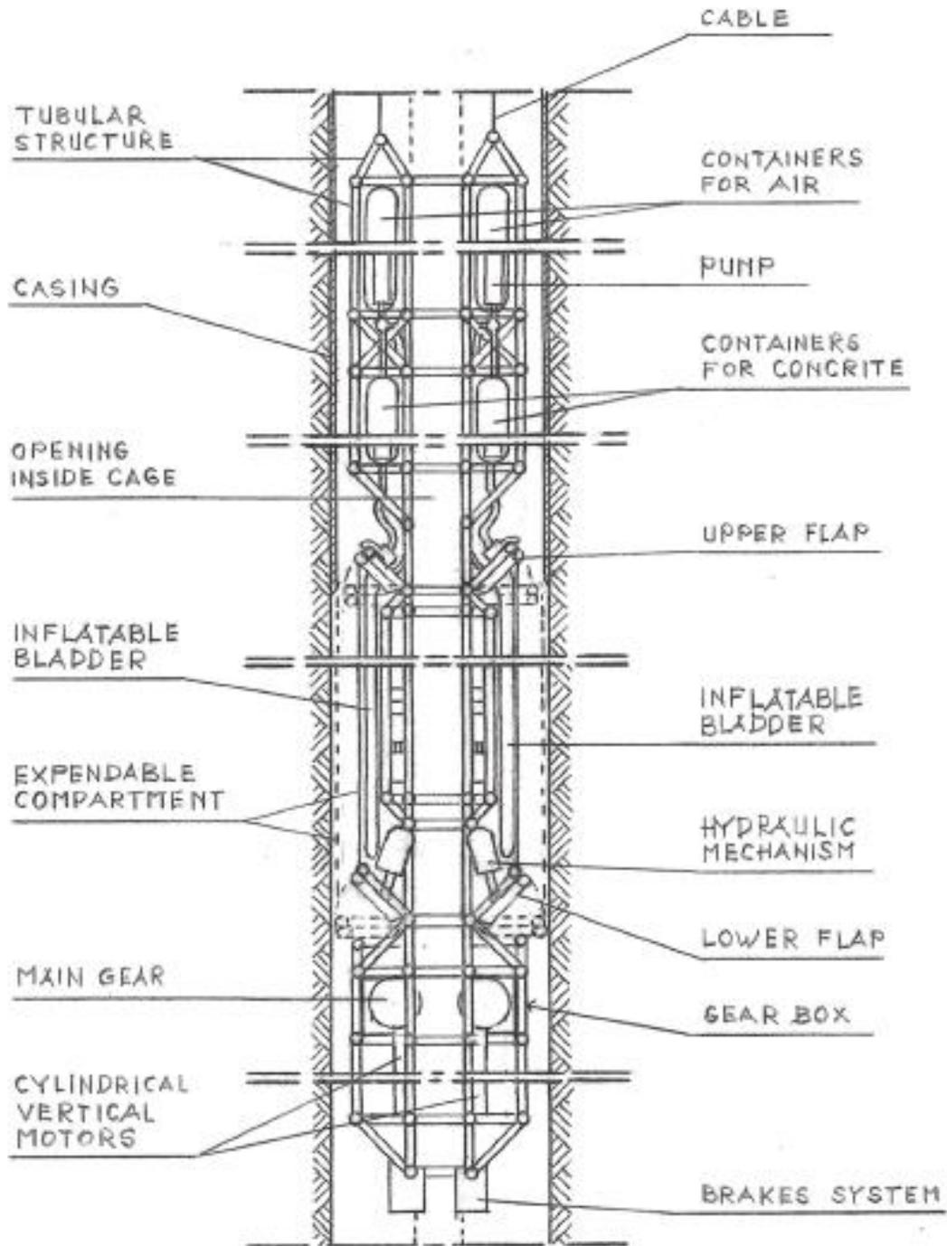
**FIG. 7** - Cross-sectional view of a circular cage to be assembled on the excavation line of the apparatus for drilling faster, deeper, and wider wellbore.
