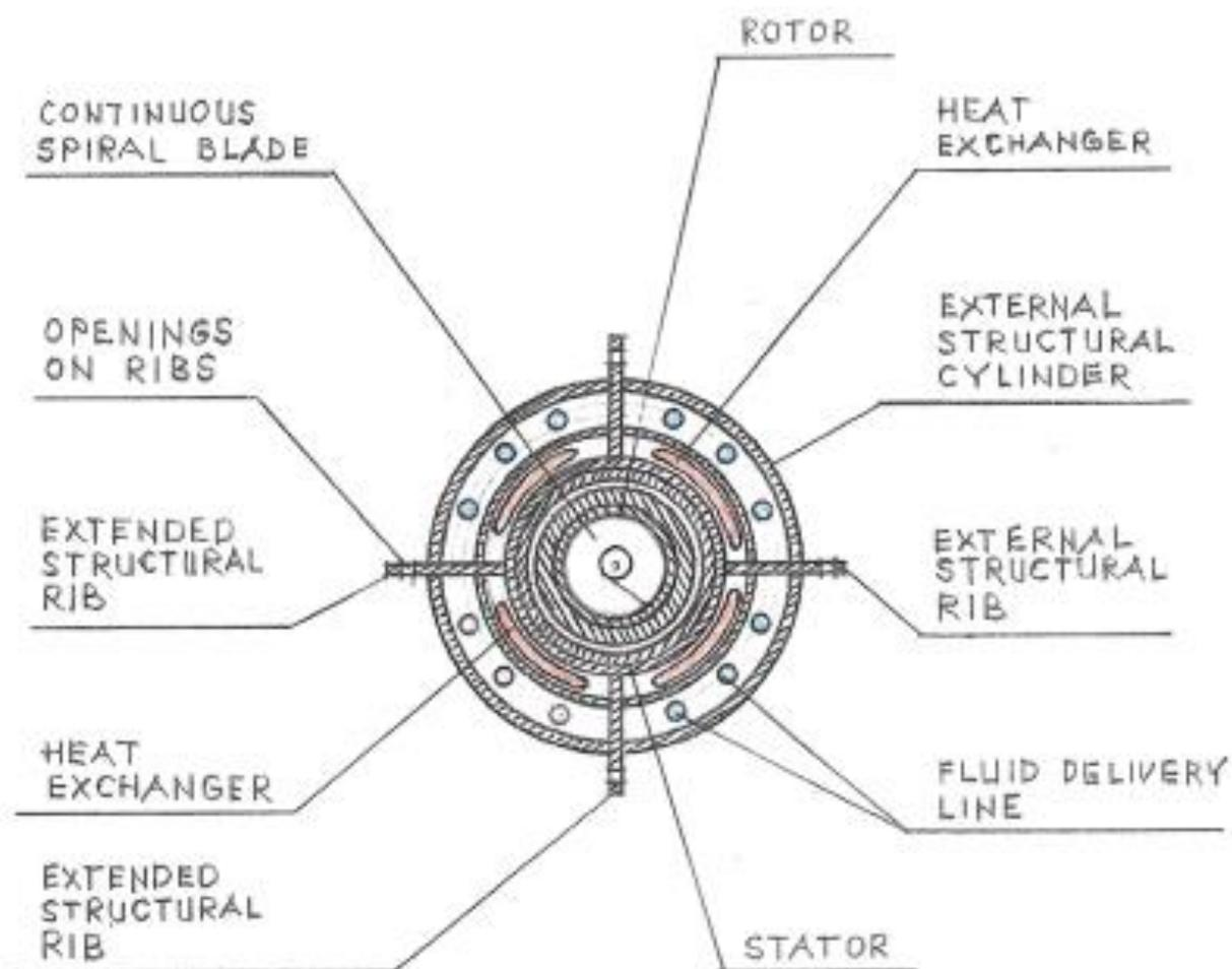
**FIG. 6** - Cross-sectional view of an excavation line of the apparatus for drilling faster, deeper, and wider wellbore.
