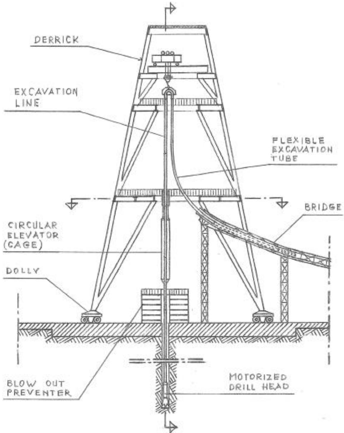
**FIG. 3** - Another schematic view of an apparatus for drilling faster, deeper and wider wellbore with cage for casing.
