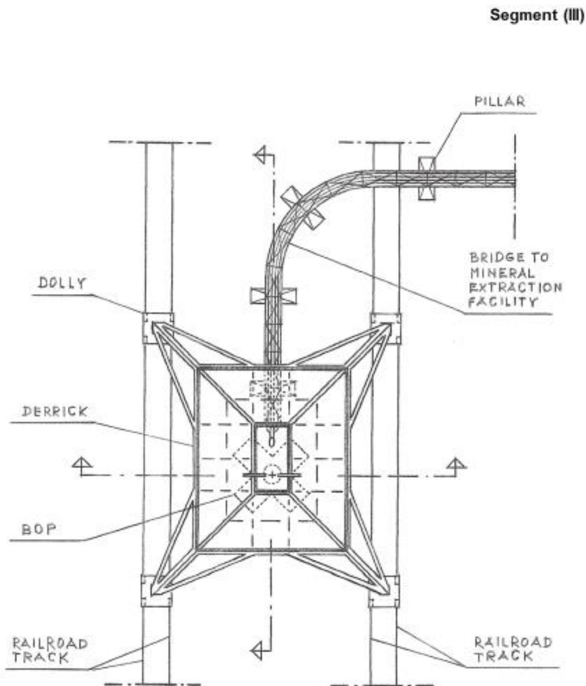
**FIG. 4** - Plain cross-sectional view of an apparatus for drilling faster, deeper and wider wellbore.
